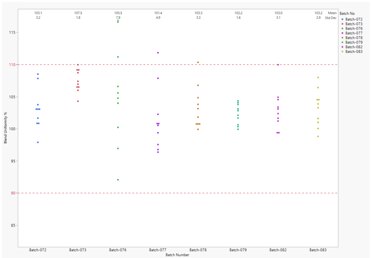
Figure 53: Comparison of small scale and pilot scale batches expressed as BU% LC mean and %RSD
