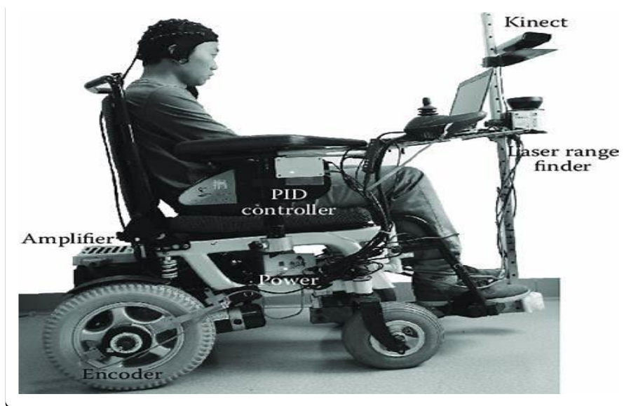
Figure 4: An intelligent wheelchair based on a BCI and an autonomous navigation system (Pan and Li, 2018)
